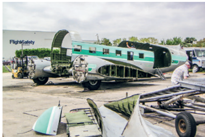
Den stormskadade N2401 demonteras i West Palm.
