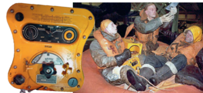
SCR-578 Gibson Girl Emergency Transmitter
